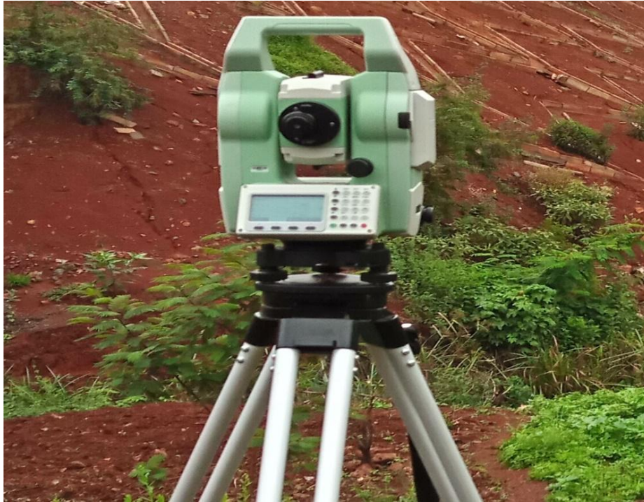
Figure 1: A total station in use in one of the previous projects.
